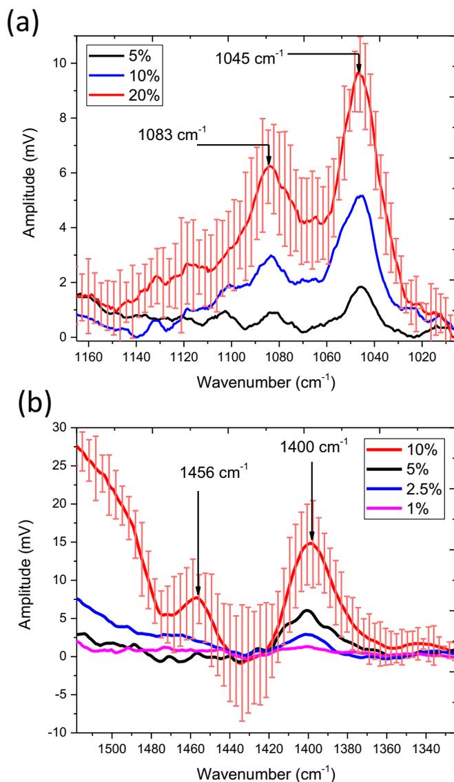
**Figure 2.** Nanomechanical IR spectrum of different concentrations of (a) ethanol-water mixtures. (b) ampicillin sodium salt, measured by using bi-material microchannel cantilever (BMC). Different colors show different analyte concentrations. For both types of the samples, the amplitude of absorption peaks relate linearly to the concentration of the solutions. The data has been plotted after smoothing using a Savitzky–Golay filter. (Adapted from our previous work.<sup>28</sup>)
