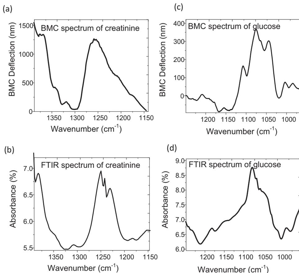
**Figure 3.** A BMC is irradiated with two different QCLs to produce nanomechanical IR spectra of (a) 110mM of creatinine sample (c) 5.4 mM of glucose. For comparison, the FTIR spectroscopy is performed for (b) 110mM of creatinine sample (d) 5.4 mM of glucose. Photothermal spectroscopy using the BMC is based upon measurement of localized heat generation while FTIR follows Lambert-Beer Law.
